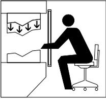
Hazardous machine parts can only be reached after passing through the protection field.
