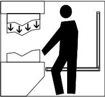
The presence of staff members between the protection field and hazardous machine parts must be prevented/avoided (protection against stepping over).
