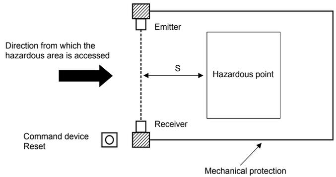
The formulae and calculation examples are related to the vertical set-up (refer to drawing) of the AOPD with regard to the hazardous point. Please observe the applicable harmonised EN standards and possible applicable national regulations.
