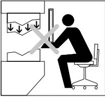
Hazardous machine parts can be reached without passing through the protection field.
