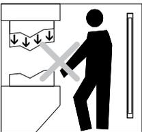
The presence of staff members between the protection field and hazardous machine parts is possible.
