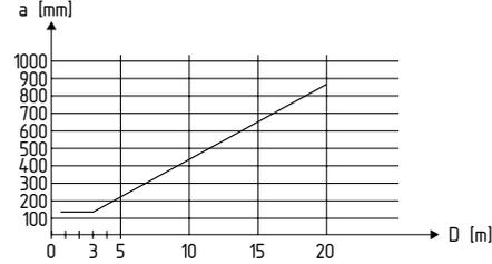
Calculate the minimum distance to reflecting surfaces as a function of the distance with an aperture angles of  $\pm 2.5^\circ$  degrees or use the value from the table below:
