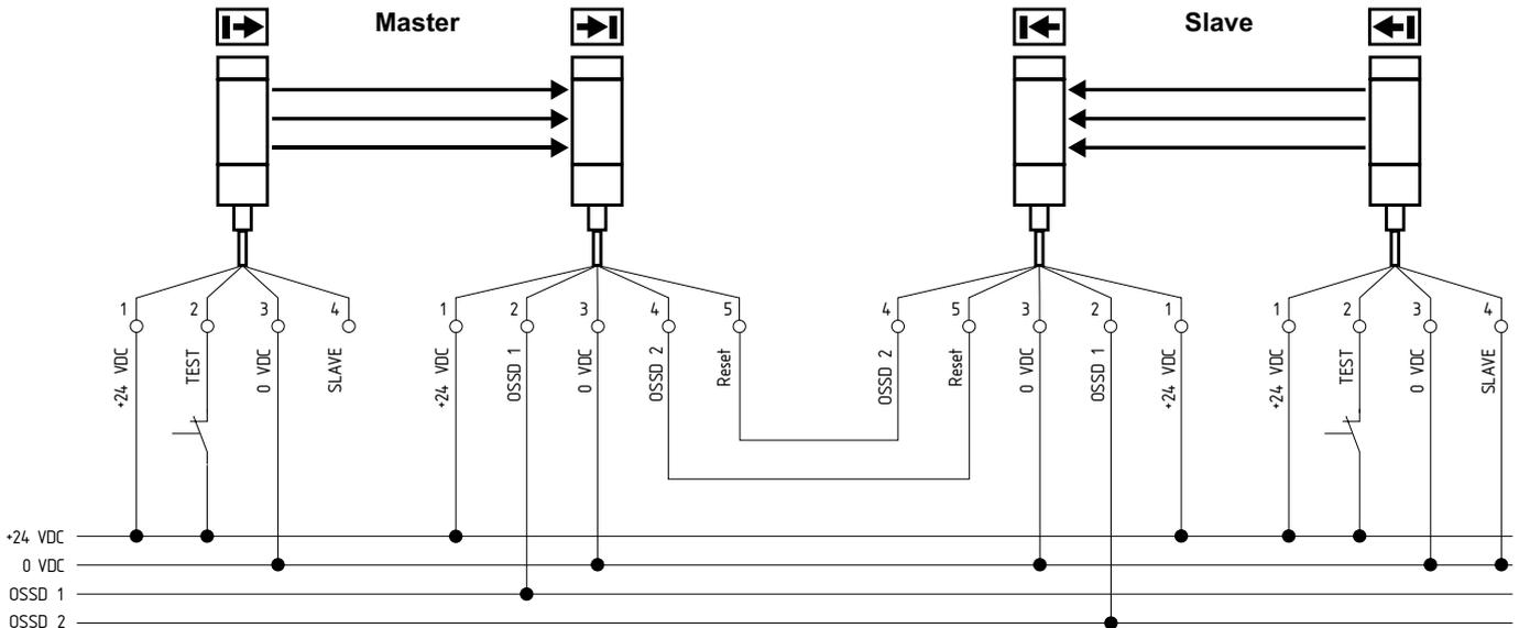
4.3 Wiring example with safety-monitor module
