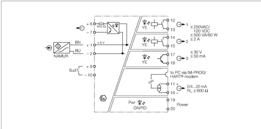
The rotation speed monitor IM21-14EX-CDTRI monitors frequencies, rotation speeds and pulse trains of rotating motor, gear or turbine parts according to over or undershoot of adjusted limit values. The current value is indicated on a display on the front of the device.
