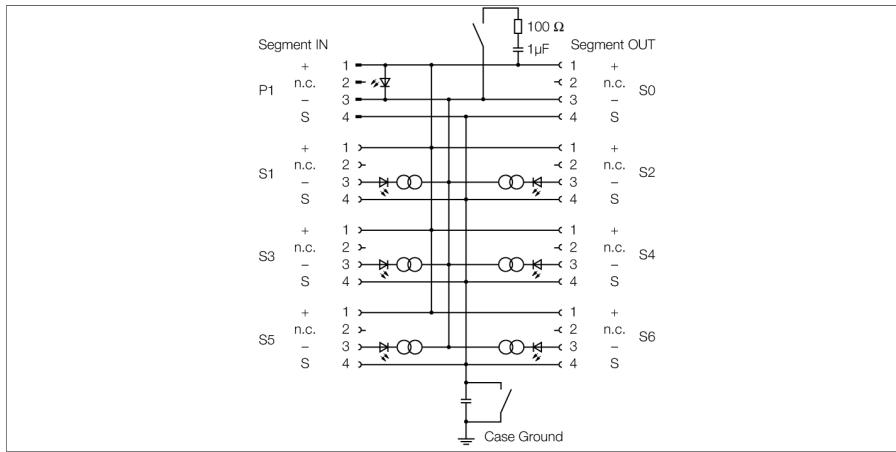
The 6-channel Ex junction box JBBS-48SC-M613/EX is designed for PROFIBUS-PA systems.
