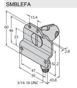
Mounting bracket, rotatable, stainless steel, for sensors of the LE250/550 series
