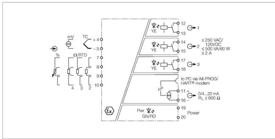
The 1-channel Ex-area temperature measuring amplifier IM34-14Ex-CDRI is designed to evaluate the temperature-dependent changes of Ni100/Pt100 RTDs and thermocouples types B, E, J, K, L, N, R, S, T and to output them as temperature-linear current signals 0/4...20 mA. Furthermore, resistors, potentiometers or low voltages can be mapped linearly as current signals in a range between -160...+160 mV.
