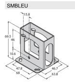
3086755 Protective housing, stainless steel, for sensors of the LE250/550 series
