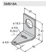
3033200 Mounting bracket, rectangular, stainless steel, for sensors with 18 mm thread
