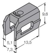
Mounting bracket for mounting magnetic field sensors on dovetail groove cylinders; groove width: 7.35 mm; material: PPS
