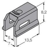
Mounting bracket for mounting magnetic field sensors on dovetail groove cylinders; groove width: 7 mm; material: PPS
