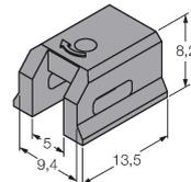
Mounting bracket for mounting magnetic field sensors on dovetail groove cylinders; groove width: 9.4 mm; material: PPS
