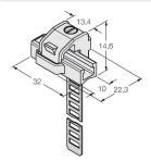
Mounting bracket for mounting magnetic field sensors on round cylinders; cylinder diameter: 25...63 mm; material: PA 6I/6T / nickel silver; fire-hazard classification acc. to UL94 - V2
