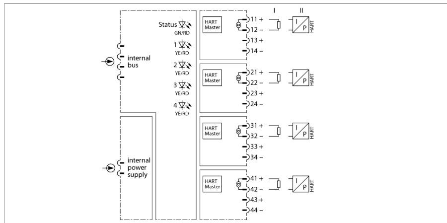
The output module AOH401-N is designed for the connection of analog actuators such as control valves or process indicators.
