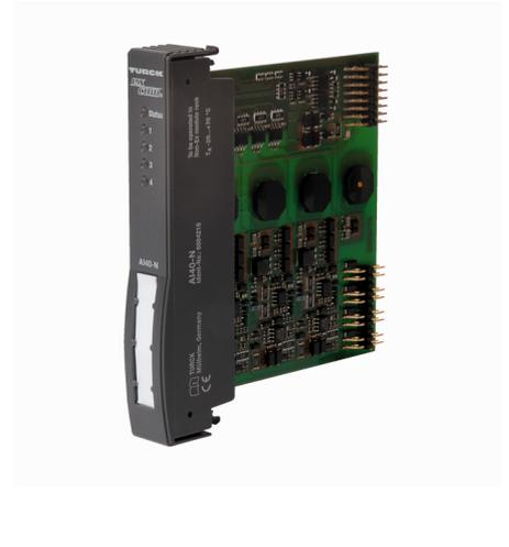
The input module AI40-N is used for the connection of 2-wire transducers (active input = source mode / transducer passive) or 4-wire transducers (passive input = sink mode / transducer active).
