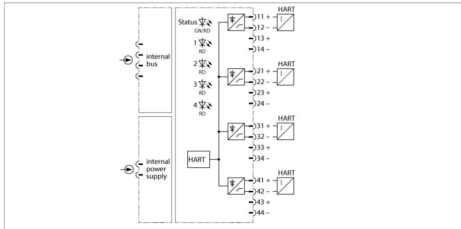
The input module AIH40-N is used for the connection of 2-wire transducers (active input = source mode / transducer passive).
