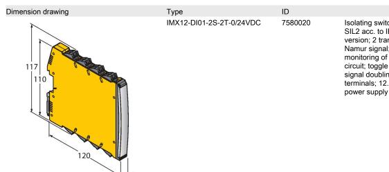
Isolating switching amplifier, 2-channel; SIL2 acc. to IEC 61508; Ex-proof version; 2 transistor outputs; input Namur signal; ON/OFF switchable monitoring of wire-break and short-circuit; toggle between NO/NC mode; signal doubling; removable screw terminals; 12.5 mm wide; 24 VDC nower supply
