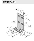
Mounting bracket, for PVA and PVD, stainless steel; set consisting of two brackets and screws
