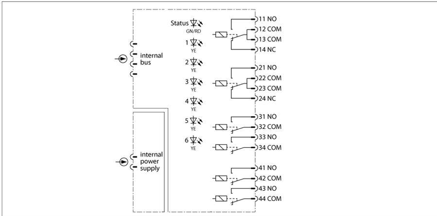
The relay module DO60R-N is used for the connection of non-intrinsically safe actuators such as valves or indicator lights.
