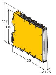
Isolating transducer; 2-channel; power supply of passive 2-wire isolating transducers with HART communication as well as connection of active 2-wire transmitters, SIL2 acc. to IEC61508; Ex-proof version; selectable with either current source/sink or voltage output; removable screw terminals; 24 VDC power supply
