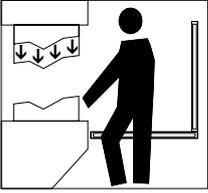
Persons between the protection field and hazardous machine parts must be prevented (protection against stepping over).
