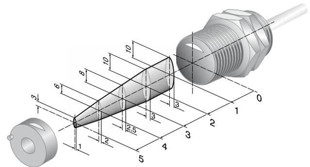
Assured switching distance:  $S_{ao} = 5 \text{ mm}$
